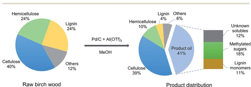
Fig. 2 Composition of birch wood, the carbohydrate residue and product oil mixture after reductive fractionation over a tandem Al(OTf)<sub>3</sub> and Pd/C catalyst system. (Reaction conditions: 2000 mg of extracted birch wood sawdust (125–300 μm), 200 mg of 5 wt% Pd/C, 15 mg of Al(OTf)<sub>3</sub>, 40 ml of methanol, 30 bar H<sub>2</sub>, stirring speed: 500 rpm, 2 h.)
