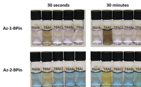
Fig. 3 Photograph of test solutions of **Az-1-Bpin** and **Az-2-Bpin** upon exposure to tetra-*n*-butylammonium halides in THF. In each solution, [analyte] = 180  $\mu\text{M}$ , which for TBAF corresponds to 3.4  $\text{mg L}^{-1}$  of fluoride anion. (For absorption spectra, see Fig. S1 in the ESI†).
