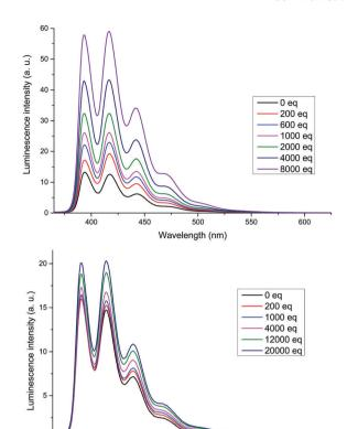
Fig. 4 Emission spectra of 3b (top) and 4b (bottom) titrated with TBABr. Host concentration: 1 μM in CHCl<sub>3</sub> (3b) or 1:1 CHCl<sub>3</sub>/acetone **(4b)**,  $\lambda_{ex} = 350 \text{ nm}$ .
