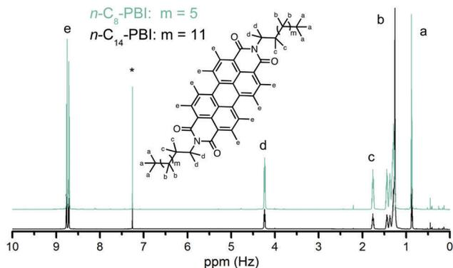
Fig. 3  $^1\text{H-NMR}$  spectra (600 MHz,  $\text{CDCl}_3/\text{TFA}$ : 5/1 v/v, 16 scans) of  $n\text{-C}_n\text{-PBI}$ s synthesized hydrothermally at  $200\text{ }^\circ\text{C}$  for 24 h; black =  $n\text{-C}_{14}\text{-PBI}$ , turquoise =  $n\text{-C}_8\text{-PBI}$ . Solvent residual peak (7.26 ppm) is marked with \*.
