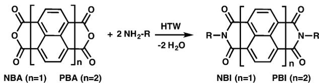
Fig. 1 Hydrothermal condensations of NBIs and PBIs: the dianhydrides NBA and PBA are reacted with different monoamines in equimolar ratio (1 : 2, no excess of  $\text{RNH}_2$ ). HTW = high-temperature water, here: 200 °C and autogenous pressure.
