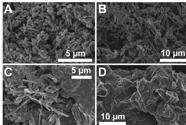
Fig. 2 SEM images of hydrothermally synthesized PBIs and PBA. (A) Hydrothermally treated PBA (24 h, 200 °C). (B–D)  $n\text{-C}_n\text{-PBIs}$  obtained hydrothermally (24 h, 200 °C). B =  $n\text{-C}_5\text{-PBI}$ , C =  $n\text{-C}_8\text{-PBI}$ , D =  $n\text{-C}_{12}\text{-PBI}$ .
