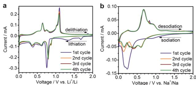
Fig. 3 Cyclic voltammograms of SnSb NCs tested in (a) Li-ion or (b) Na-ion half-cells using a scan rate of  $0.1 \text{ mV s}^{-1}$  in the potential range of 0.005–2.0 V.
