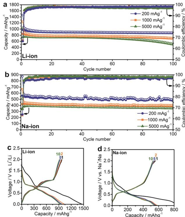
Fig. 2 Electrochemical performance of SnSb NCs. Capacity retention of SnSb NCs in (a) Li-ion and (b) Na-ion half-cells at currents of 200, 1000 and 5000  $\text{mA g}^{-1}$ . Galvanostatic charge and discharge curves of SnSb NCs in (c) Li-ion and (d) Na-ion half-cells at a current of 200  $\text{mA g}^{-1}$ . All measurements were performed in the potential range of 0.005–2.0 V.
