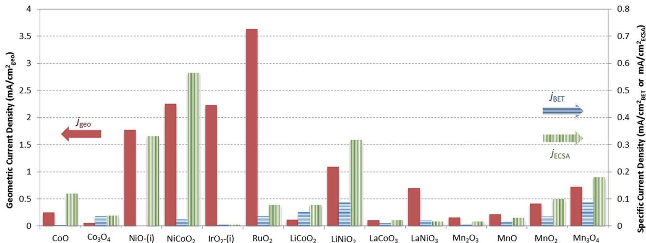
Fig. 5 The current density per geometric surface area (red), and specific current densities per BET surface area (blue) and ECSA (green) at 0.35 V overpotential in 1 M NaOH. Due to the large difference between the measured geometric and specific current densities for most systems, two scales are used as shown in the figure, with the geometric current density plotted against the scale to the left, and the specific current density per BET and ECSA is plotted with the scale on the right.
