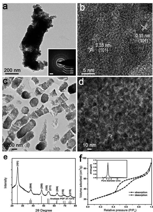
Fig. 2 Characterization of nanostructured anatase 5-TiO<sub>2</sub> annealed under air. (a) TEM image and corresponding SAED (inset) of representative rod-shaped structure. Scale bar in the inset is 2 nm<sup>-1</sup>. (b) HRTEM image of the rod-shaped structure. (c) Low and (d) high magnification microtome TEM images of anatase. (e) XRD pattern of nanostructured anatase. (f) Nitrogen adsorption and desorption isotherms and pore size distribution (inset).
