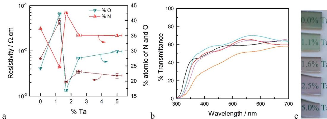
Fig. 1 (a) Resistivity (brown) and atomic% of O (blue) and N (red) of Ta-doped TiO<sub>2</sub> as a function of % Ta. (b) Optical transmittance of Ta-doped TiO<sub>2</sub> films, un-doped TiO<sub>2</sub> (orange), 5.0% Ta (black), 2.5% Ta (red), 1.67% Ta (cyan) and 1.25% Ta (pink). (c) Photographs of the TTO films after annealing in ammonia at 750 °C for 30 min.
