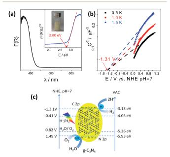
Fig. 1 (a) UV-vis DRS spectrum of  $g-C_3N_4$  polymers; inset: the corresponding Tauc plot. (b) Mott–Schottky plots of the  $g-C_3N_4$  electrode in 0.2 M Na<sub>2</sub>SO<sub>4</sub>, pH = 7. (c) Band structure diagram of  $g-C_3N_4$  polymers calculated by optical absorption and typical electrochemical Mott–Schottky methods.
