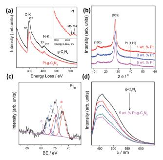
Fig. 3 (a) EELS of the  $g-C_3N_4$  polymers with Pt deposited *in situ*. (b) XRD of the  $g-C_3N_4$  polymers with Pt deposited *in situ*. (c) High resolution of XPS analysis of Pt<sub>4f</sub>. (d) PL spectra of the  $g-C_3N_4$  polymers with Pt deposited *in situ*.
