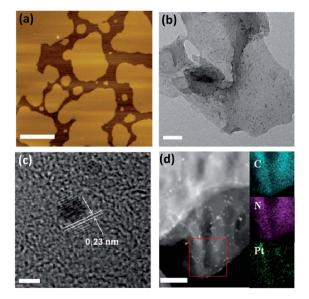
Fig. 2 (a) AFM image of the  $g-C_3N_4$  polymers with Pt deposited *in situ*. (b) TEM image of the  $g-C_3N_4$  polymers with Pt deposited *in situ*. (c) HR-TEM image of the  $g-C_3N_4$  polymers with Pt deposited *in situ*. (d) STEM images of the  $g-C_3N_4$  polymers with Pt deposited *in situ*. Scale bar for a, b, c and d is 50 nm, 100 nm, 2 nm and 50 nm, respectively.
