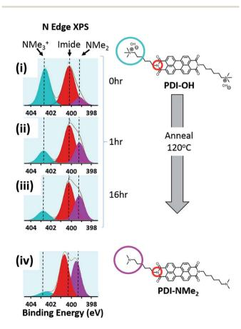
**Fig. 2** Conversion of NMe $_3$ <sup>+</sup> to NMe $_2$  in PDI-OH proceeds upon thin film annealing at 120 °C ((i) 0 h, (ii) 1 h, (iii) 16 h) as observed *via* XPS (N 1s spectra). As expected, after extended annealing, the XPS spectrum of films of PDI-OH closely resembles that of PDI-NMe $_2$  (iv).
