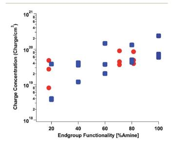
Fig. 3 Electron paramagnetic resonance (EPR). Quantitative measurements of charge carrier concentration in PDI samples were done in triplicate for all samples: (1) PDI-NMe<sub>2</sub>/PDI-C6 composites with varying PDI-NMe<sub>2</sub> content (blue squares), (2) annealed PDI-OH samples (red circles). Error bars for each measurement are on the scale of the data points.
