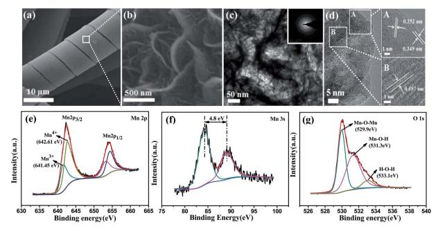
Fig. 1 (a and b) SEM images of the helical  $Na_xMnO_2$  with hierarchical porous structures; (c) TEM and (d) HRTEM images of the typical  $Na_xMnO_2$  nanosheets (inset in (c) is the SAED pattern); XPS spectra of the helical  $Na_xMnO_2$  of (e) Mn 2p, (f) Mn 3s, and (g) O 1s.
