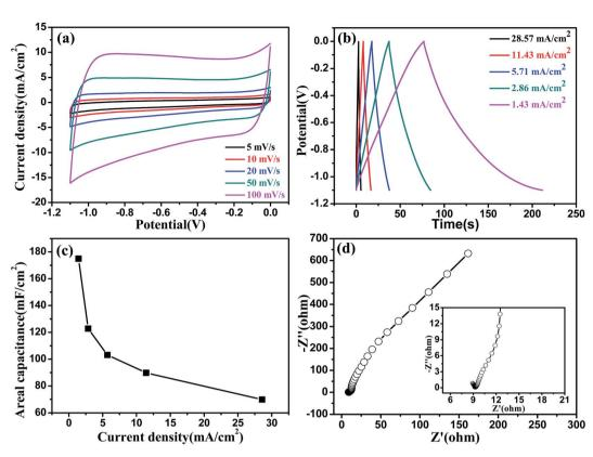
Fig. 4 (a) CV curves at different scan rates; (b) GCD curves at different current densities of the helical MoO<sub>2</sub> in 1.0 M Na<sub>2</sub>SO<sub>4</sub> electrolyte; (c) areal capacitance calculated from GCD curves as a function of current densities; (d) EIS spectra of MoO2 (inset is the enlarged view of the high frequency region).
