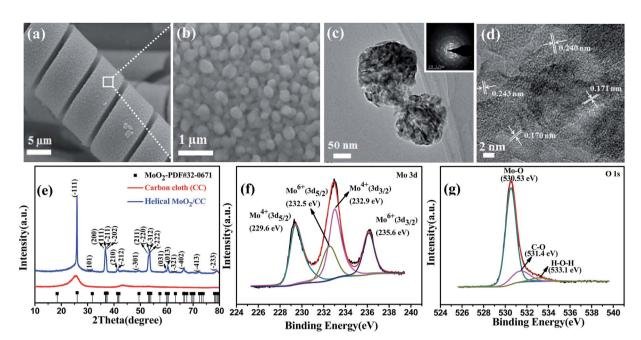
Fig. 3 (a and b) SEM images of the helical MoO<sub>2</sub> with different magnifications; (c) the TEM image of MoO<sub>2</sub> nanoparticles (inset is the SAED pattern); (d) the HRTEM image of the helical MoO<sub>2</sub>; (e) XRD patterns of the helical MoO<sub>2</sub>/CC and CC; XPS spectra of the helical MoO<sub>2</sub>/CC: (f) Mo 3d and (a) O 1s.
