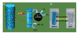
Fig. 8 (a) Schematic illustration for the photocatalytic degradation of MB on TiO<sub>2</sub>-wsCQDs composite under UV light irradiation and (b) digital images of MB before and after degradation.
