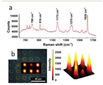
Fig. 7 SERRS detection of Crystal Violet on an array of GNR supercrystals coated with mesoporous silica. (a) Typical SERRS spectra of CV measured on the supercrystals. (b) SERRS signal obtained by mapping the SERRS intensity of the crystal violet vibrational peak over 1618–1632 cm<sup>-1</sup>, as observed in a Raman microscope and reconstructed in three dimensions with intensity given as height.
