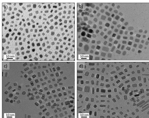
**Fig. 8** TEM image of Pt nanocrystals obtained under the non-aqueous route with CO–liquid segmented flow. OAm/OLA = 3.8, Pco = 120 psi and residence time = 150 s: (a) 200 °C, and OLA/Pt = 45 molar ratio; (b) 200 °C and OLA/Pt = 150 molar ratio; (c) 215 °C, OLA/Pt = 150 molar ratio; (d) 230 °C, OLA/Pt = 150 molar ratio.
