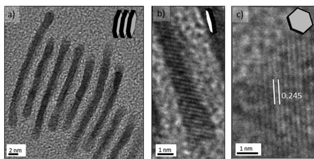
**Fig. 5** HRTEM images of the palladium nanosheets synthesized under CO–liquid segmented flow at 90 °C in 150 s; liquid segments contain DMF and TTABr: (a) stack of palladium sheets perpendicular to the HRTEM grid; (b) lattice fringes from the nanosheet edge; (c) lattice fringes of a nanosheet lying flat on the TEM grid.
