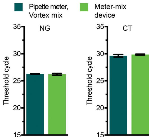
Fig. 4 qPCR threshold cycles on DNA extracted from urine spiked with either inactivated *Chlamydia trachomatis* (CT) or *Neisseria gonorrhoeae* (NG). Sample metering and mixing with lysis buffer was performed with either the meter-mix device (light green bars) or standard pipette and vortex (dark green bars). The remainder of the extraction protocol was identical for both conditions.
