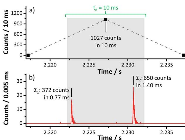
**Fig. 4** Transient signal of 30 nm AuNP ( $C_{\text{NP}} = 2.5 \times 10^5$  NP mL<sup>-1</sup>) simultaneously acquired with ICP-MS software (a) and the home-built DAQ (b) for 20 ms. A potential problem in single particle ICP-MS due to particle coincidence within one dwell time is observed in (a) because two individual transient events occurred during one dwell time (grey rectangle indicates a 10 ms dwell time interval used in the ICP-MS software).
