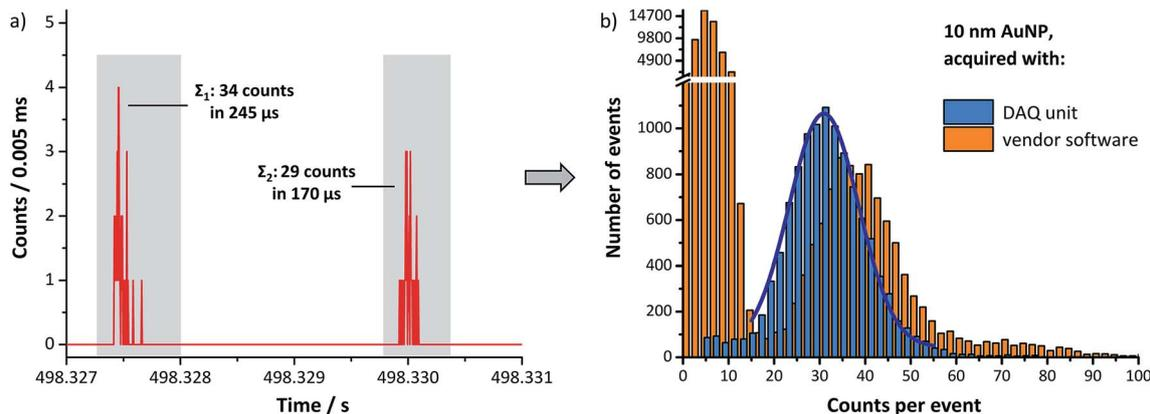
Fig. 6 (a) Representative ICP-MS signal due to two single 10 nm-sized AuNPs ( $C_{\text{NP}} = 5 \times 10^5 \text{ NP mL}^{-1}$ ) acquired with the home-built DAQ for 4 ms (counts per 5  $\mu\text{s}$  for individual signal pulses identified as individual events). (b) Corresponding intensity histograms of 10 nm-sized AuNPs simultaneously acquired with ICP-MS software (orange) and the home-built DAQ (blue) for 600 s.
