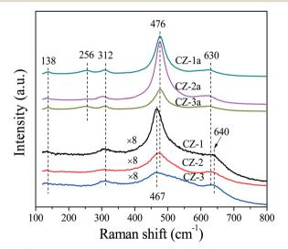
Fig. 2 Raman spectra of fresh and aged Ce<sub>0.5</sub>Zr<sub>0.5</sub>O<sub>2</sub> samples.
