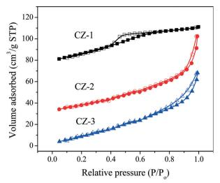
Fig. 3 Nitrogen adsorption/desorption isotherms of fresh Ce<sub>0.5</sub>Zr<sub>0.5</sub>O<sub>2</sub> samples prepared with different methods.
