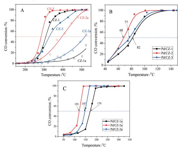
Fig. 10 Conversion of CO over (A) fresh and aged CZ, (B) fresh and (C) aged 1 wt% Pd/CZ (1000 ppm CO + 20% O<sub>2</sub>/Ar, GHSV of 30 000 h<sup>-1</sup>).
