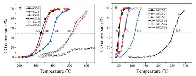
Fig. 11 Conversion of CO over (A) fresh and aged CZ, (B) fresh and aged 1 wt% Pd/CZ (1000 ppm CO + 20% O<sub>2</sub> + 5% H<sub>2</sub>O/Ar, GHSV of 30 000 h<sup>-1</sup>).
