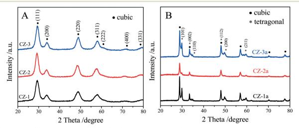
Fig. 1 XRD patterns of (A) fresh and (B) aged Ce<sub>0.5</sub>Zr<sub>0.5</sub>O<sub>2</sub> solid solutions prepared by different methods
