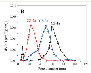
Fig. 4 Pore diameter distribution curves of (A) fresh and (B) aged Ce<sub>0.5</sub>Zr<sub>0.5</sub>O<sub>2</sub> samples prepared with different methods
