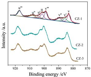
Fig. 5 Ce 3d XPS spectra of the Ce<sub>0.5</sub>Zr<sub>0.5</sub>O<sub>2</sub> samples prepared by different methods.
