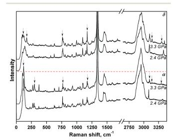
Fig. 4 Raman spectra of the  $\alpha$ - and  $\delta$ -polymorphs of chlorpropamide providing evidence of the phase transitions in the pressure change from 2.4 to 3.3 GPa. The most significant changes in the Raman spectra are shown by arrows and are mainly related to lattice vibrations (50–350 cm<sup>-1</sup>), CC and SO stretching vibrations (750–1250 cm<sup>-1</sup>) and rearrangements of H-bonds (3050–3360 cm<sup>-1</sup>).
