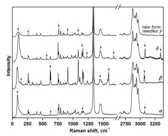
Fig. 3 Raman spectra of the  $\alpha$ -,  $\beta$ -, and  $\delta$ -polymorphs of chlorpropamide and the new needle-shaped (y) polymorph at the first pressure point (0.3 GPa). No solid-state transformations occur in the starting  $\alpha$ and  $\delta$ -forms at this pressure. Characteristic features of the spectra for the different polymorphs are shown by arrows.
