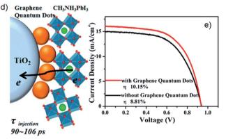
**Fig. 8** (a) Schematic of GQD structure. (b) Energy levels of different layers used in PSCs of Zhu *et al.*, <sup>81</sup> (c) Cross sectional SEM image of PSCs fabricated with GQDs. (d) Schematic illustration of electron generation and injection at the interfaces of TiO<sub>2</sub>, GQDs and perovskites. (e) Current density–voltage curves for the best performing PSCs. Reprinted with permission from ref. 81 © 2014, American Chemical Society.
