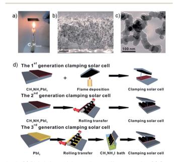
Fig. 5 (a) Digital photo of the candle-soot film preparation. (b) Cross sectional SEM image of the candle-soot film. (c) TEM image of the asprepared candle-soot particles. (d) Fabrication processes of the candle-soot film based PSCs. Reprinted from ref. 70.
