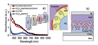
Fig. 7 (a) UV-vis spectra of P<sub>3</sub>HT and perovskite films with and without C<sub>60</sub>SAM. Inset: the energy level of the components used in Snaith's work.85 (b) The structure of the PSC fabricated with C<sub>60</sub>SAM layer between perovskite and TiO<sub>2</sub> layers. Reprinted with permission from ref. 85 © 2013, American Chemical Society.
