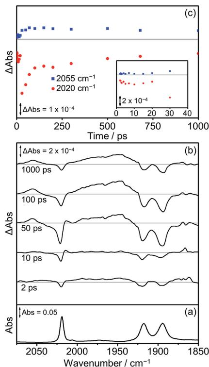
Fig. 12 FTIR and TRIR spectra of **Dyad 3 Br** in THF: (a) FTIR ground state spectrum; (b) TRIR difference spectra taken 2, 10, 50, 100 and 1000 ps after flash photolysis at 560 nm; (c) TRIR single point kinetic traces for the ground state bands (red dots, 2020  $\text{cm}^{-1}$ ) and the  $^3\text{MLCT}$  excited state (blue squares, 2055  $\text{cm}^{-1}$ ). Inset shows expansion of the first 40 ps.
