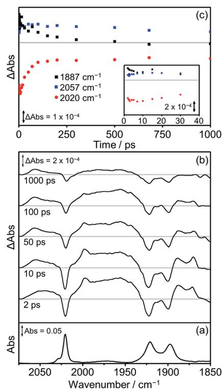
Fig. 11 FTIR and TRIR spectra of **Dyad 2 Br** in THF: (a) FTIR ground state spectrum; (b) TRIR difference spectra taken between 2, 10, 50, 100 and 1000 ps after flash photolysis at 560 nm; (c) TRIR single point kinetic traces for the CS product (black squares, 1887  $\text{cm}^{-1}$ ), the ground state bands (red dots, 2020  $\text{cm}^{-1}$ ) and the <sup>3</sup>MLCT excited state (blue squares, 2057  $\text{cm}^{-1}$ ). Inset shows expansion of the first 40 ps.
