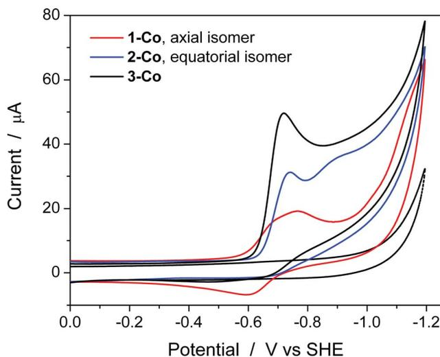
Fig. 4 Aqueous cyclic voltammometry of catalysts **1-Co** (red), **2-Co** (blue), and **3-Co** (black) in 1 M pH 7 KPBS at glassy carbon electrode. Catalyst concentration is 1 mM and scan rate = 100 mV s<sup>-1</sup>. Background is shown as a dotted gray line.
