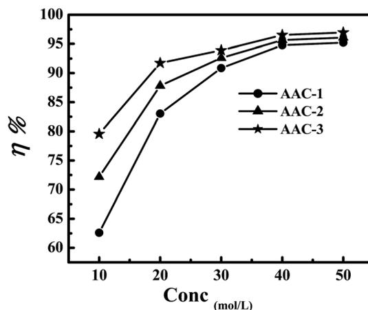
Fig. 2 Variation of inhibition efficiency with AACs concentration.
