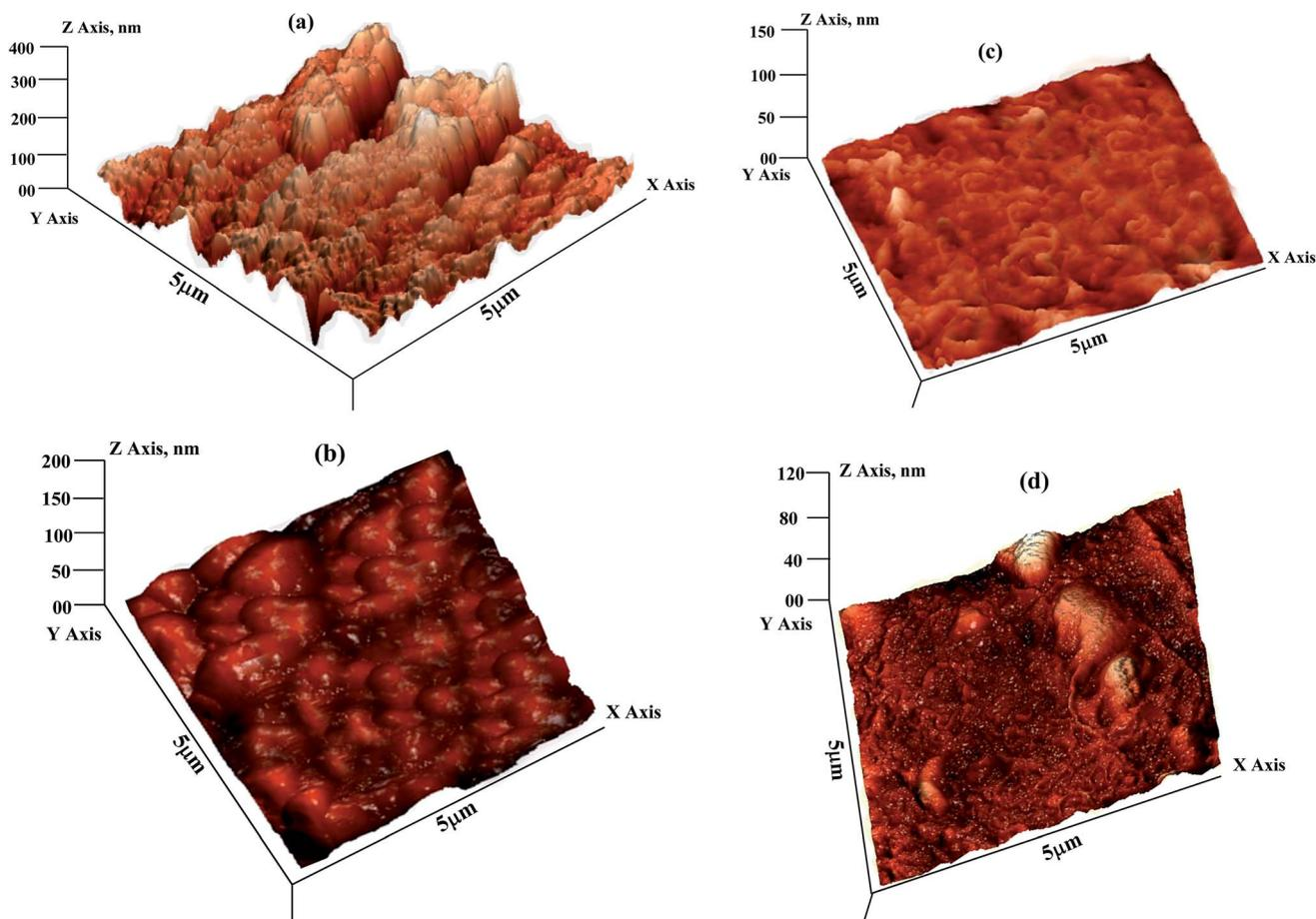
**Fig. 10** (a–d) AFM images of mild steel: (a) in absence of AACs and in the presence of 40 mg L<sup>-1</sup> of (b) AAC-1, (c) AAC-2, and (d) AAC-3.
