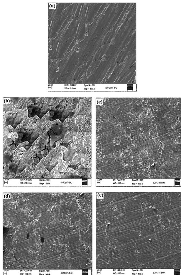
Fig. 8 (a–e) SEM images of mild steel surfaces: (a) abraded, (b) in absence of AACs and in the presence of  $40 \text{ mg L}^{-1}$  of (c) AAC-1, (d) AAC-2, and (e) AAC-3.
