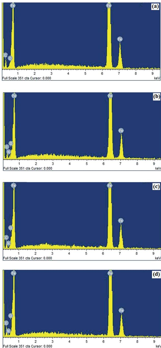
Fig. 9 (a–d) EDX images of mild steel: (a) in absence of AACs and in the presence of 40 mg L<sup>-1</sup> of (b) AAC-1, (c) AAC-2, and (d) AAC-3.
