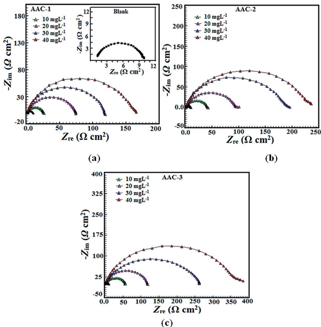
Fig. 6 (a–c) Nyquist plot for mild steel in 1 M HCl without and with different concentrations of AACs.
