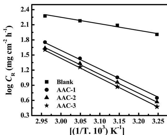
**Fig. 3** Arrhenius plots for the corrosion rate of mild steel versus the temperature in 1 M HCl.**Table 4** Values of activation energies for mild steel dissolution in 1 M HCl in the absence and at of optimum concentration of AACs
