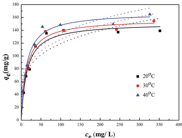
Fig. 9 Langmuir isotherm (solid line) and Freundlich isotherm (dash line) for the adsorption of Cr(vi) on CMB (reaction conditions:  $c_0 = 20\text{--}500$   $\text{mg L}^{-1}$ ;  $V = 50$   $\text{mL}$ ;  $m = 50$   $\text{mg}$ ;  $t = 6$   $\text{h}$ ;  $\text{pH} = 2$ ;  $T = 20, 30, 40$   $^\circ\text{C}$ ).
