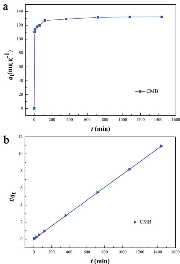
**Fig. 10** (a) Effect of contact time of Cr(vi) adsorption onto CMB and (b) pseudo-second-order sorption kinetics of Cr(vi) adsorption onto CMB (reaction conditions:  $c_0 = 200 \text{ mg L}^{-1}$ ;  $V = 50 \text{ mL}$ ;  $m = 50 \text{ mg}$ ;  $\text{pH} = 2$ ;  $T = 30 \text{ }^\circ\text{C}$ ).
