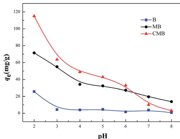
Fig. 8 Effect of the initial solution pH on adsorption of Cr(vi) by B, MB and CMB (reaction conditions:  $c_0 = 150 \text{ mg L}^{-1}$ ;  $V = 50 \text{ mL}$ ;  $m = 50 \text{ mg}$ ;  $t = 6 \text{ h}$ ;  $T = 30 \text{ }^\circ\text{C}$ ).
