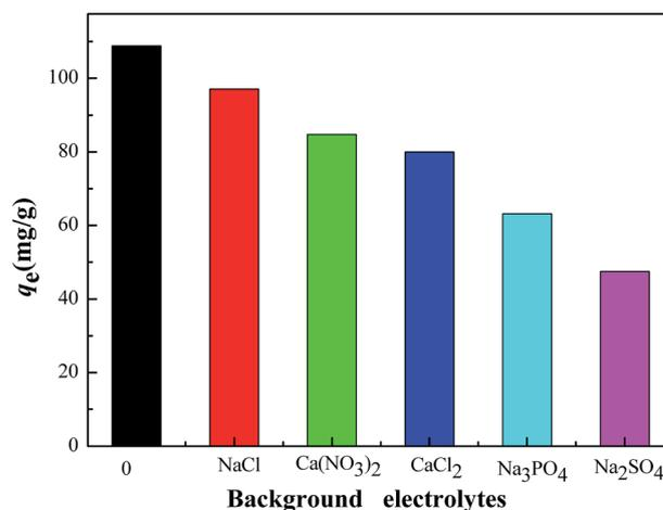
**Fig. 11** Effect of background electrolyte (NaCl, Ca(NO<sub>3</sub>)<sub>2</sub>, CaCl<sub>2</sub>, Na<sub>3</sub>PO<sub>4</sub>, Na<sub>2</sub>SO<sub>4</sub>) on the Cr(vi) adsorption by CMB. (Reaction conditions: electrolyte concentration 0.01 mol L<sup>-1</sup>; Cr(vi) concentration  $c_0 = 150 \text{ mg L}^{-1}$ ;  $V = 50 \text{ mL}$ ;  $m = 50 \text{ mg}$ ;  $T = 30 \text{ }^\circ\text{C}$ ;  $\text{pH} = 2$ ).
