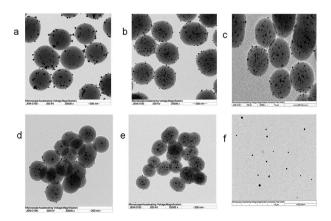
**Fig. 9** TEM images, with 200 nm scale bar, of different sizes of polydopamine spheres loaded with silver nanoparticles (Ag@PDS) controlled by adjusting the amount of aqueous ammonia: (a) 1.0 ml, (b) 1.25 ml, (c) 1.5 ml, (d) 1.75 ml, (e) 2.0 ml and (f) pure Ag NPs. Ag@PDS of different sizes are applied in the antibacterial experiments.
