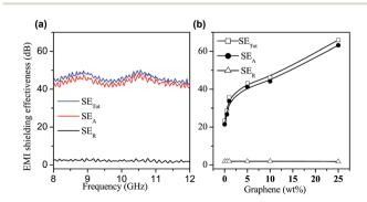
Fig. 3 (a) The comparison between  $SE_{Tot}$ ,  $SE_R$  and  $SE_A$  for the graphene/PEDOT:PSS sample with 10% graphene loading, and (b) the same for samples with different graphene loadings at 10 GHz.
