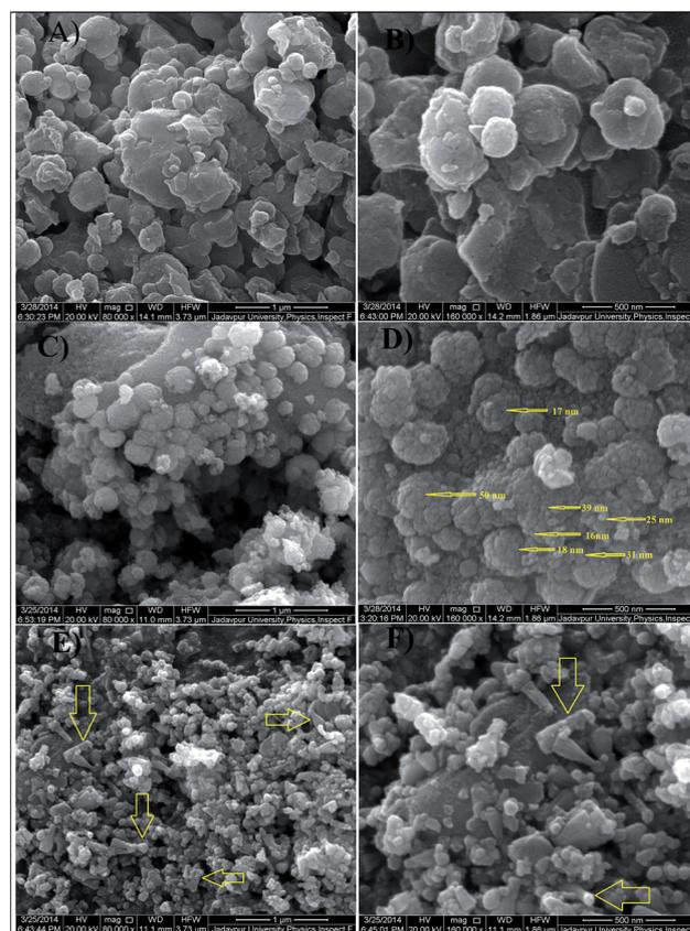
Fig. 3 FESEM micrograph of synthesized ZnO. (A) PZN30 at 1  $\mu\text{m}$  scale; (B) PZN30 at 500 nm scale; for PZN60 particles were spherical in nature and each particle was aggregation of many smaller particles. (C) PZN60 at 1  $\mu\text{m}$  scale; (D) PZN60 at 500 nm scale. For PZN100 dumbbell shaped larger particles due to crystal growth. (E) PZN100 at 1  $\mu\text{m}$  scale; (F) PZN100 at 500 nm scale.
