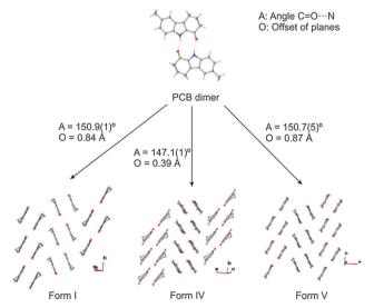
Fig. 3 Crystal packing of the three polymorphs of PCB as determined by single-crystal X-ray diffraction.
