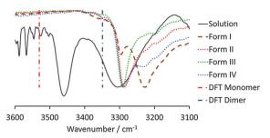
Fig. 2 N-H region of the normalised transmission FTIR spectra of a 0.542 M solution of OCB in chloroform and the four crystal forms. Vertical lines depict the DFT-calculated N-H vibrations of the monomer and dimer.
