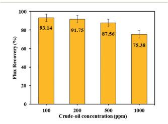
Fig. 10 Flux recovery rate of PES/HMO-2 membrane at different oil concentrations in the feed.
