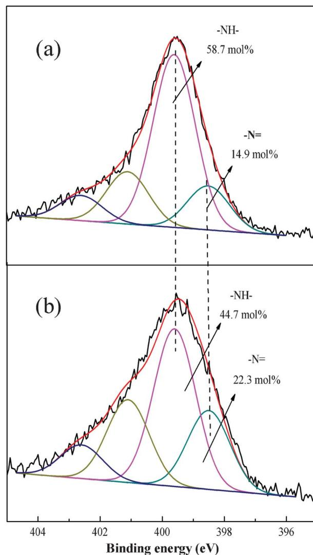
Fig. 13 N 1s core level spectra of PAN/PANI nanofiber mat before (a) and after (b) Cr(vi) adsorption.
