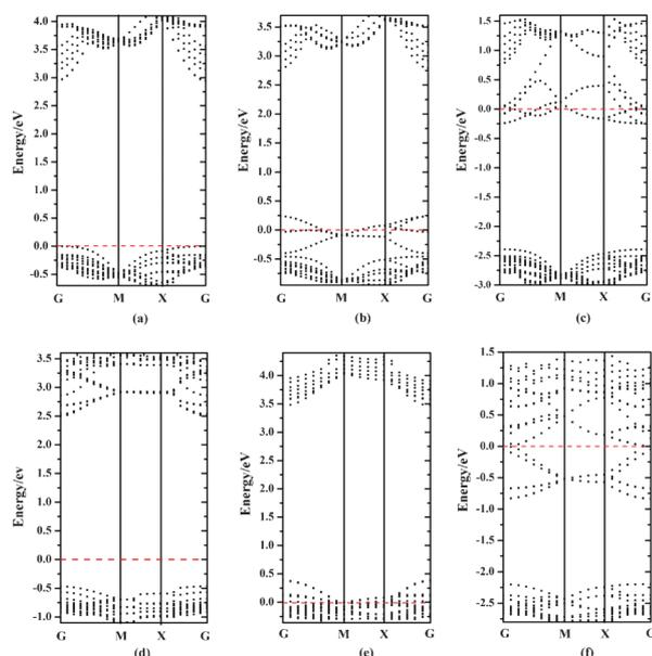
**Fig. 2** (a–c) Band structures of 1-layer F, 2-layer F and BiO terminated {001} facets for BiOF, respectively. (e) and (f) are band structures of O and BiF terminated {110} BiOF facets, respectively. (d) represents the band structure of the BiOF with {010} facet. Red dashed lines represent the Fermi level at 0 eV.
