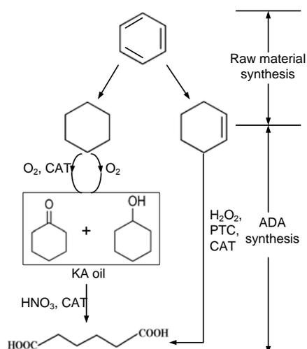
Scheme 1: Two-(left) and one-step (right) production routes of adipic acid<sup>83</sup> reprinted with permission from Elsevier.
