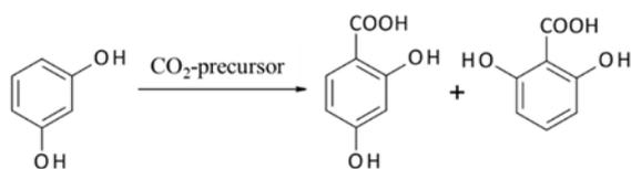
Scheme 5: Kolbe-Schmitt synthesis starting from resorcinol with a CO<sub>2</sub>-precursor giving 2,4 DHBA (target product) and 2,6 DHBA as by-product (Krtschil *et al.*<sup>107</sup>).
