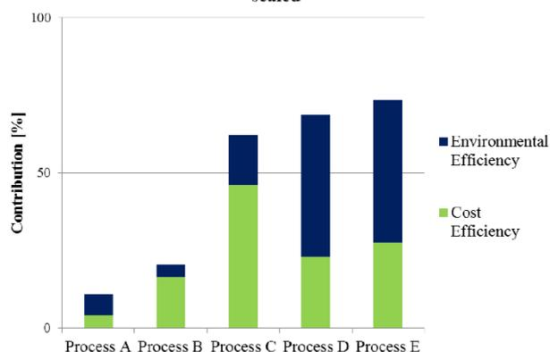
Figure 7: Criteria contribution (scaled) to overall eco-efficiency ranking of different biodiesel production alternatives utilising waste oil (Process A: pre-treated alkali-catalysed; Process B: acid-catalysed; Process C: heterogeneous acid-catalysed; Process D: supercritical process, Process E: supercritical, microreactor based process) according to Kralisch *et al.*<sup>72</sup>
