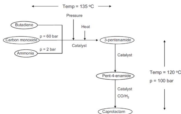
Figure 11: Flow sheet for the novel catalytic production of caprolactam studied by LCA<sup>79</sup> reprinted with permission from Elsevier.
