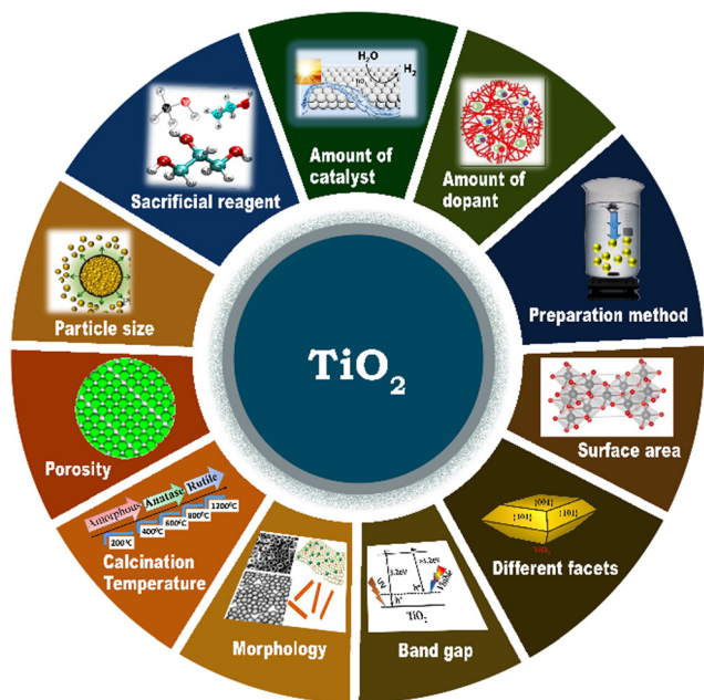
Fig. 15 Schematic representation of the various factors that determine the photocatalytic hydrogen evolution activity of TiO 2 -based photocatalysts.
