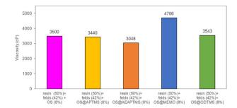
**Fig. 4** Viscosity values for the mixtures resin/feldspar/OS@silanized (50/42/8 %w/w). All the measurements were performed in triplicate (Table S7†).
