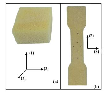
Compressive (a) and tensile (b) foam samples
