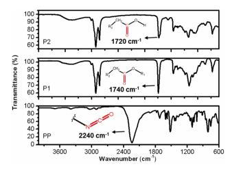
Fig. 11 FT-IR spectra from the polyurethane precursors.
