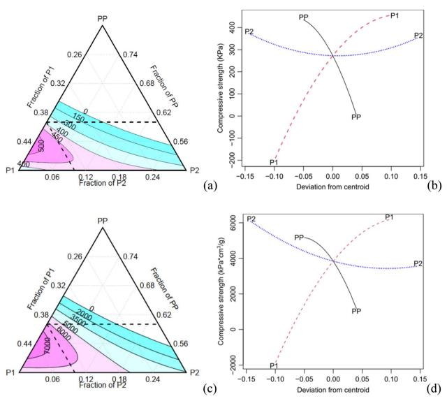
Contour and effect (plots: (a, b) absolute and(c, d) specific compressive strength.
