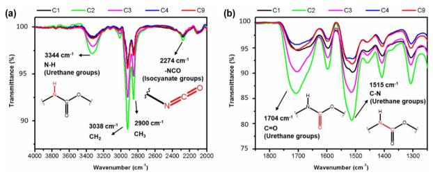
Fig. 14 FT-IR spectra of from 4000-2000 cm<sup>-1</sup> (a) and from 1900 to 1200 cm<sup>-1</sup> (b) indicating the different extents of urethane linkages formation within the samples
