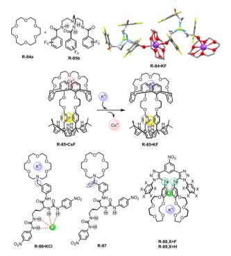
Fig. 24 Chemical structure of the receptors R-84 to R-89 with ion-pair binding and crystal structures of R-84·KF (data from the Cambridge Crystallographic Data Centre [CCDC # 732760]).<sup>115</sup>
