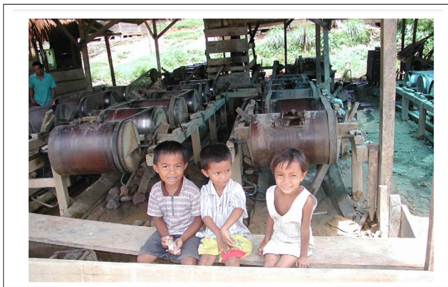
Fig. 2 Miners in Sulawesi, Indonesia, add one kilogram of mercury to each ball mill when kids play nearby the operational area. Reproduced with permission from ref. 38, copyright 2024, J. Clean. Prod.
