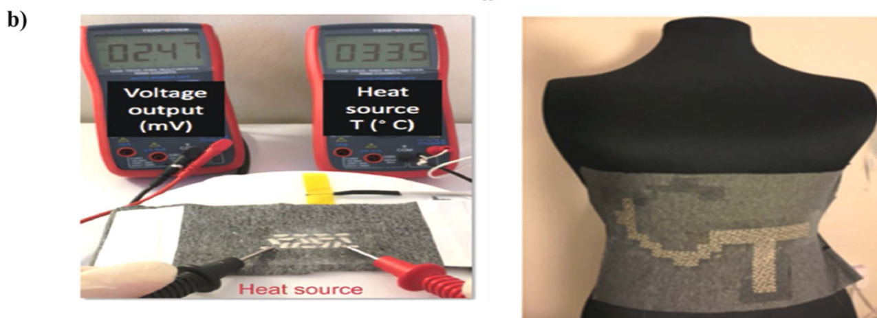
Fig. 27 (a) PEDOT:PSS-based textile TE generator (49). (b) Textile-integrated polymer-based TE generator (50).
