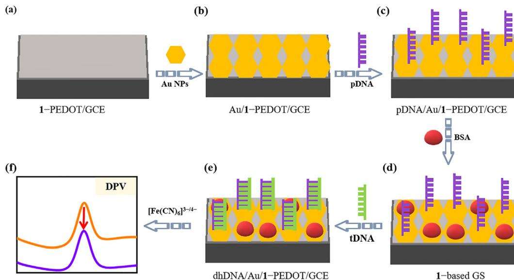
**Scheme 2** Mechanism of detecting the  $\beta$ -thalassemia gene by the 1-based GS: (a) the 1-PEDOT film modified GCE (1-PEDOT/GCE); (b) Au deposited 1-PEDOT/GCE (Au/1-PEDOT/GCE); (c) pDNA grafted Au/1-PEDOT/GCE (pDNA/Au/1-PEDOT/GCE); (d) BSA-treated pDNA/Au/1-PEDOT/GCE (1-based GS); (e) 1-based GS capturing tDNA (dhDNA/Au/1-PEDOT/GCE); (f) DPV response of dhDNA/Au/1-PEDOT/GCE.
