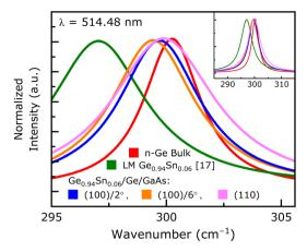
Fig. 6 Raman spectra recorded from epitaxial Ge<sub>0.94</sub>Sn<sub>0.06</sub> layers of samples A1, B2 and C (compressively strained heterostructures), selectively chosen with different orientations alongside a lattice matched Ge<sub>0.94</sub>Sn<sub>0.06</sub> epilayer.<sup>17</sup> Positive Raman wavenumber shifts (representing compressively strained states) are observed on all three samples A1: (100)/2°, B2: (100)/6°, and C: (110).
