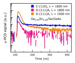
Fig. 10  $\mu$ -PCD measurement data acquired with 1800 nm excitation wavelength for samples C-(110) and D-(111)A. High surface recombination induced noisy signals make the curve inconducive to single exponential fit, with  $R^2$  fitting parameter reaching only 0.41 with 1 as the perfect fit. Similar results are observed at 1500 nm for D-(111)A orientation, indicating its high electrical conductivity, irrespective of excitation wavelength.
