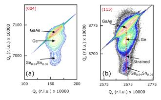
Fig. 3 Reciprocal space maps (RSMs) taken along the (a) (004) and (b) (115) orientations, that shows ~0.81% compressive strain in the 100 nm thick Ge<sub>0.94</sub>Sn<sub>0.06</sub> epitaxial layer (sample B1) grown on 27 nm Ge layer/ (100)/6° GaAs substrate.
