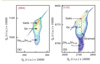
Fig. 2 Reciprocal space maps (RSMs) taken along the (a) (004) and (b) (115) orientations, that shows ~0.81% compressive strain in the 100 nm thick Ge<sub>0.94</sub>Sn<sub>0.06</sub> epitaxial layer (sample A1) grown on 27 nm Ge/(100)/ 2° GaAs substrate.
