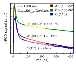
Fig. 8  $\mu$ -PCD signal *versus* time acquired at 300 K with 1500 nm excitation wavelength from samples A1 [(100)/2° Ge<sub>0.94</sub>Sn<sub>0.06</sub>], B1 [(100)/6° Ge<sub>0.94</sub>Sn<sub>0.06</sub>] and C [(110) Ge<sub>0.94</sub>Sn<sub>0.06</sub>]. The corresponding minority carrier lifetimes of ~319 ns, ~481 ns and ~434 ns were obtained by fitting to exponential decay after the initial surface recombination induced decay.
