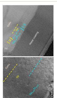
Fig. 5 Cross-sectional TEM micrographs of sample A2: (a) Ge<sub>0.94</sub>Sn<sub>0.06</sub>/ Ge/(100)/2° GaAs heterostructure representing good quality growth of 50 nm  $Ge_{0.94}Sn_{0.06}$  grown over 38 nm thick Ge layer grown on GaAs, where broken lines demarcate similar structure factored Ge and Ge<sub>0.94</sub>Sn<sub>0.06</sub> epilayers, and (b) HR-TEM micrograph affirms the fine quality of the GeSn/Ge heterostructure system.
