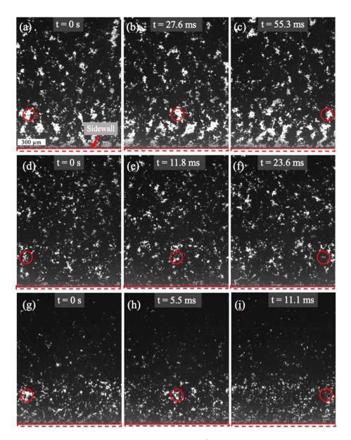
Fig. 5 Images from high-speed videos at (a-c) 35, (d-f) 50, and (g-i) 100  $\mu$ L min<sup>-1</sup> at 10x magnification with the channel sidewall at the bottom of each image, as denoted by the dashed red lines. The red circles track a void space across the width of the view field. The scale bar in (a) also applies to (b-i) and represents 300  $\mu$ m.
