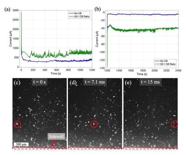
Fig. 7 (a) A comparison of the 100 μL min<sup>-1</sup> charging current with and without CB. (b) A comparison of the 100 μL min<sup>-1</sup> discharging current with and without CB. Due to the agglomeration of CB in low shear areas of the  $\mu$ -EFC, only 100  $\mu$ L min<sup>-1</sup> data could be collected. (c-e) shows still images of the carbon slurry that includes carbon black at a flowrate of 100  $\mu$ L min<sup>-1</sup>.
