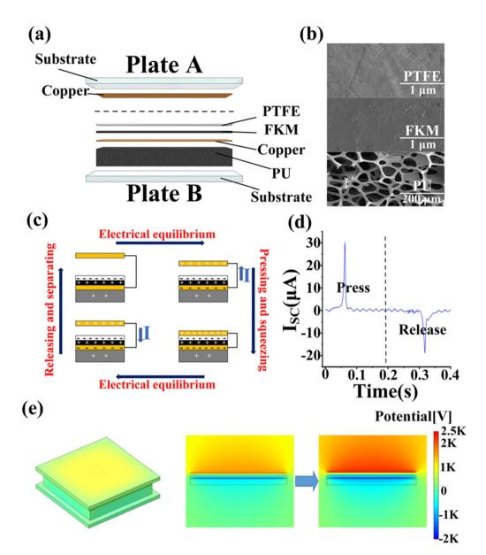
Fig. 1 (a) Internal structure and material composition of PFP-TENG. (b) The SEM of PTFE, FKM, and PU. (c) The working mechanism of PFP-TENG. (d) The  $I_{SC}$  generated in one working cycle. (e) The potential distribution simulated using COMSOL.
