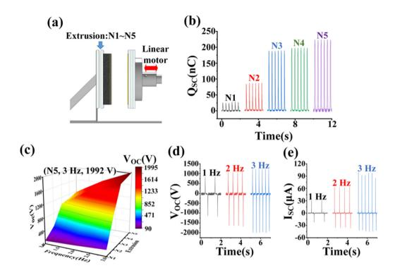
Fig. 3 (a) The working conditions of PFP-TENG. (b) The  $Q_{SC}$  values under different extrusion amounts. (c) The 3D surface graph of  $V_{OC}$  under different frequencies and extrusion amounts. The (d)  $V_{OC}$  and (e)  $I_{SC}$  changes at different frequencies.
