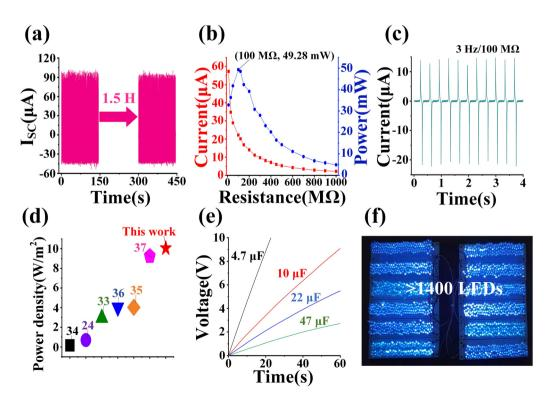
Fig. 4 (a) The reliability and (b) output power of PFP-TENG. (c) The output current at 100 M $\Omega$ . (d) Comparison of the power performance of PFP-TENG with previous designs. (e) The charging speed of difference capacitors using PFP-TENG. (f) The applicability of PFP-TENG in driving LEDs.
