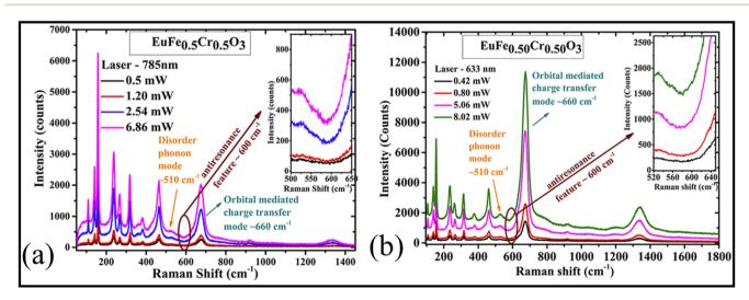
Fig. 4 Raman spectra for Cr-doped EuFeO<sub>3</sub> samples using excitation wavelengths (a) 785 nm and (b) 633 nm at different laser powers. Reproduced from ref. 49 with permission from [American Chemical Society], copyright [2022].
