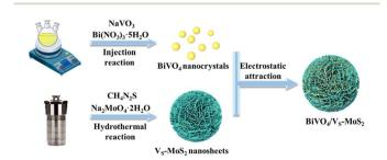
Scheme 1 Schematic illustration of the preparation process of BiVO<sub>4</sub>/  $V_S$ -MoS<sub>2</sub>.
