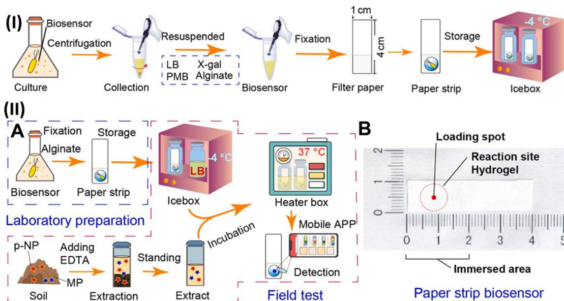
Fig. 8 (I) Schematic illustration of manufacturing of paper-strip biosensor. (II) Diagram of whole-cell biosensor device for detecting MP and *p*-nitrophenol (*p*-NP): flow-diagram of the fabrication and utilization (A) and objective drawing (B) of whole-cell paper-strip biosensor. Reproduced with permission from ref. 172 Copyright 2023, Elsevier.
