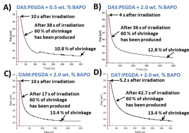
**Fig. 3** Rheometer-monitored graphs of the bio-based acrylate copolymers over time under LED light (405 nm): (A) DAS : PEGDA with 0.5 wt% of BAPO (photoinitiator); (B) DAS : PEGDA with 2 wt% of BAPO; (C) DAM : PEGDA with 2 wt% of BAPO; and (D) DAT : PEGDA with 2 wt% of BAPO. The red line indicates the time when the lamp was turned on.
