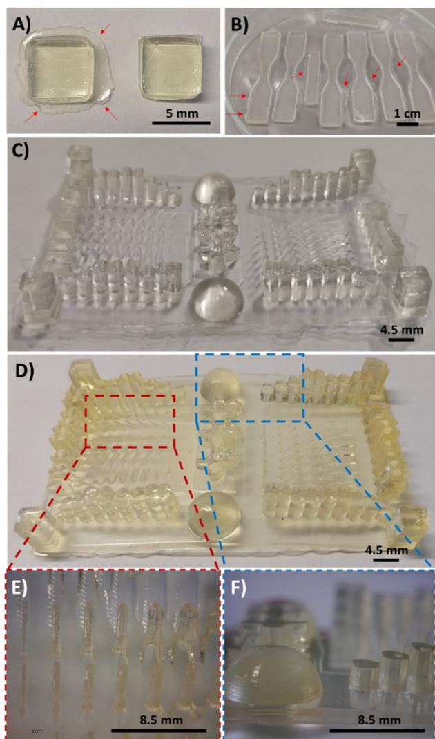
**Fig. 6** Examples of some pieces printed with the DLP 3D printer employing the bio-based resin DAS and PEGDA monomer: (A) square bar samples used for biodegradability assays. (B) Dumbbell-shaped probes for stress-strain experiments. (C) Details of the dimensional stability of the resolution piece. Arrows in (A and B) indicate the bottom membrane that can be easily removed. (D) Resolution piece after the post-curing processes. (E and F) Details from the pillars and shapes printed.
