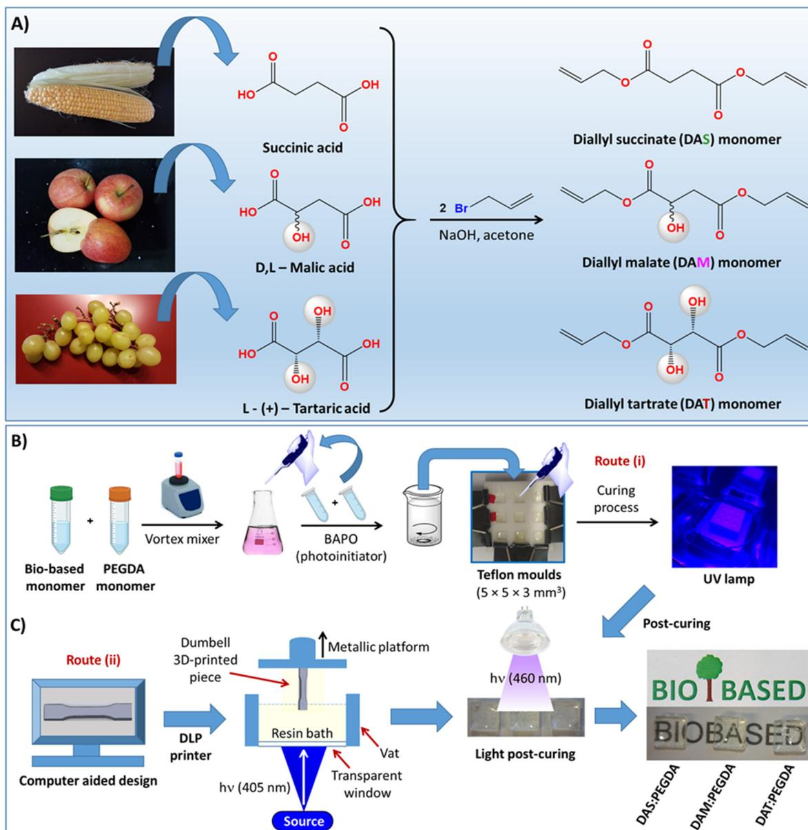
**Fig. 1** (A) Illustration of the synthetic route followed to prepare the bio-based monomers: DAS, DAM and DAT. (B) Schematic representation of the procedure carried out for the copolymerization of the bio-based monomers and PEGDA co-monomer and the subsequent deposition inside Teflon moulds and curing under light. (C) Representation of the scale-up production of dumbbell test specimens in a DLP printer and the post-curing process in controlled visible light.
