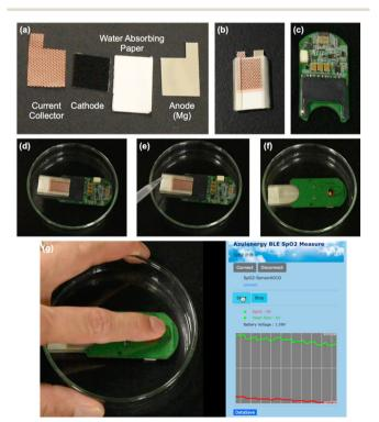
Fig. 4 Photographs of cell components (a), a single paper battery cell (b), SpO<sub>2</sub> sensor (c), SpO<sub>2</sub> sensor with the cell (d), injection of salt water to the cell (e), and the active  ${\rm SpO}_2$  sensor (other side compared with panels (d) and (e)) (f). Real-time monitoring of O2 saturation and pulse measured in a person (g).
