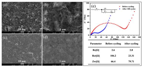
Fig. 7 FESEM images of the Fe<sub>3</sub>O<sub>4</sub> QDs@C/RGO electrode before cycling (a and b) and after 100 cycles (c and d) under various magnifications. Nyquist plots of the Fe<sub>3</sub>O<sub>4</sub> QDs@C/RGO electrode before cycling and after 100 cycles with inset showing equivalent circuit and the corresponding fitted values of the parameters (e).
