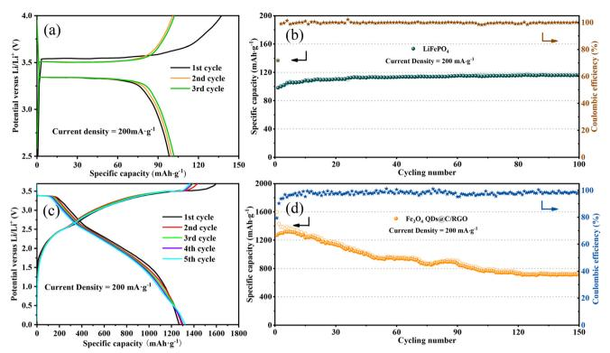
Fig. 8 Charge and discharge voltage profile (a) and cycling performance (b) of a commercial LiFePO<sub>4</sub> cathode at 200 mA  $g^{-1}$  in half cells. Charge and discharge voltage profile (c) and cycling performance (d) of the Fe<sub>3</sub>O<sub>4</sub> QDs@C/RGO sample in Fe<sub>3</sub>O<sub>4</sub> QDs@C/RGO//LiFePO<sub>4</sub> full cells at 200 mA  $g^{-1}$ .
