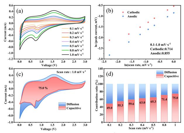
Fig. 5 CV curves of the  $Fe_3O_4$  QDs@C/RGO composite electrode from 0.1 to 1.0 mV s<sup>-1</sup> (a), the  $\ln(i)$ - $\ln(v)$  plot (b), the capacitive contribution of the  $Fe_3O_4$  QDs@C/RGO composite electrode at 1 mV s<sup>-1</sup> (c) and the pseudocapacitive contribution ratios at different scanning rates (d).
