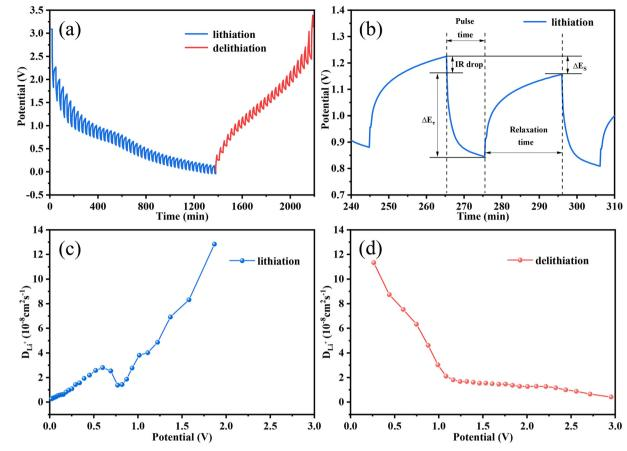
Fig. 6 GITT curves (a) and a profile for a single GITT test (b), and variation of the  $D_{\text{Li}^+}$  values during lithiation (c) and delithiation (d) processes of the Fe<sub>3</sub>O<sub>4</sub> QDs@C/RGO electrode.
