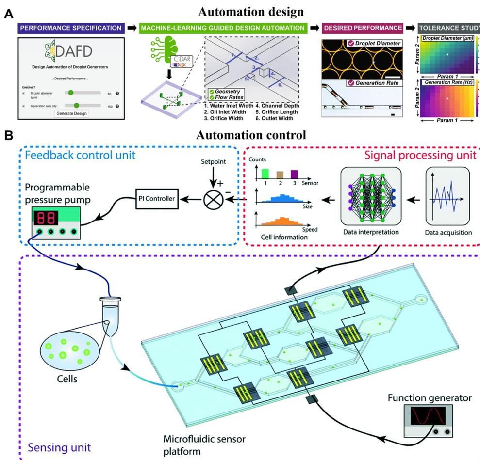
**Fig. 8** AI-accelerated high-throughput microfluidic systems with intelligent design and control. A) Machine-learning-empowered design automation for the control of microfluidic droplet generation. Reproduced from ref. 189 with permission from Springer Nature.<sup>189</sup> B) Closed-loop feedback control of microfluidic cell manipulation *via* deep-learning integrated sensor networks. Reproduced from The Royal Society of Chemistry.<sup>195</sup>
