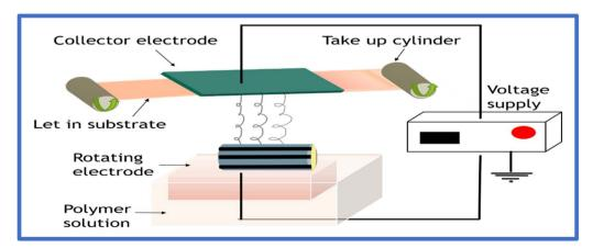
Fig. 5 Needleless electrospinning of polymeric solution.
