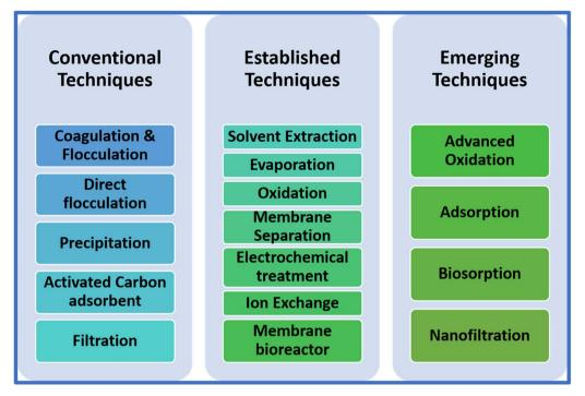
Classification of different technologies involved in effluent treatment. Reproduced with permission from ref. 52. Copyright 2022, Elsevier.
