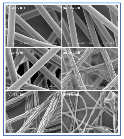
Fig. 6 Scanning electron microscopy images of electrospun nanofibers at various relative humidity. Replicated with permission from ref. 94. Copyright 2009, the American Chemical Society.
