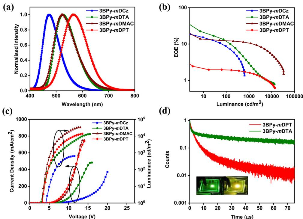
Fig. 5 (a) EL spectra; (b) EQE versus luminance characteristics (c) luminance–voltage–current density characteristics. (d) Transient EL spectra; inset is an EL illumination image of **3BPpy-mDTA** (green emission) and **3BPpy-mDPT** (yellow emission).
